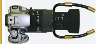
Features a superior system that includes fiber-optic lateral and medial lighting for better iris fiber definition.
